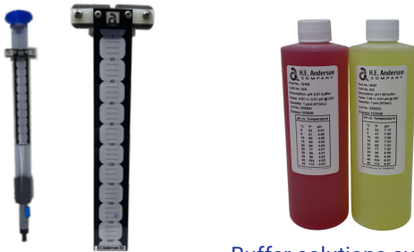
Calibration Pipe and Scale
